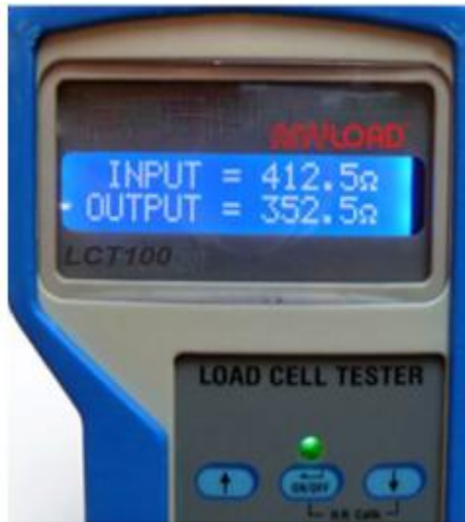
Figure 3 Typical bridge input/output results
