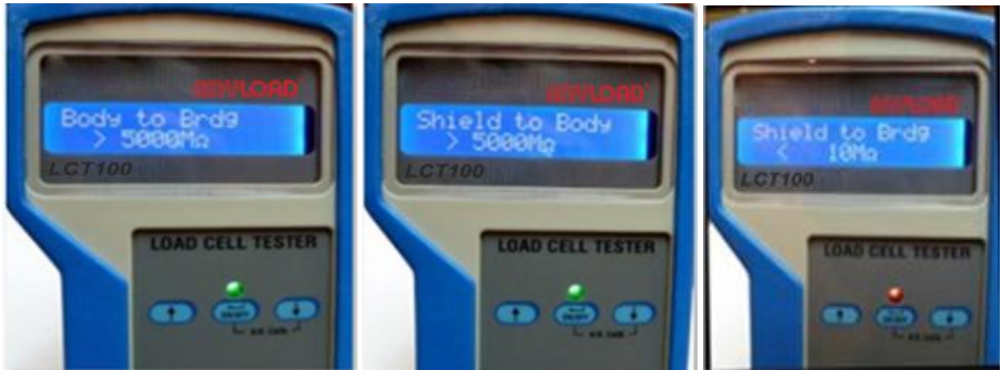
Figure 4 showing the insulation resistance results. The right one is an example of bad result and led turns red
