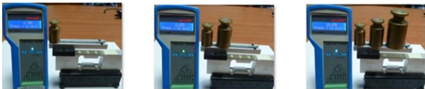
Figure 6 performing a linearity test with 3 weights
