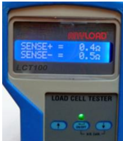
Figure 7 Typical reading when sense lines are OK
