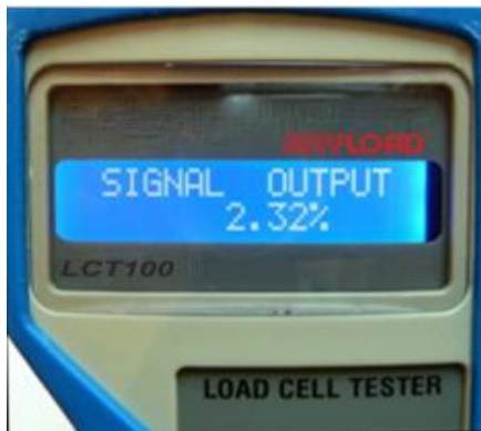
Figure 2 Zero output when load cell is loaded
